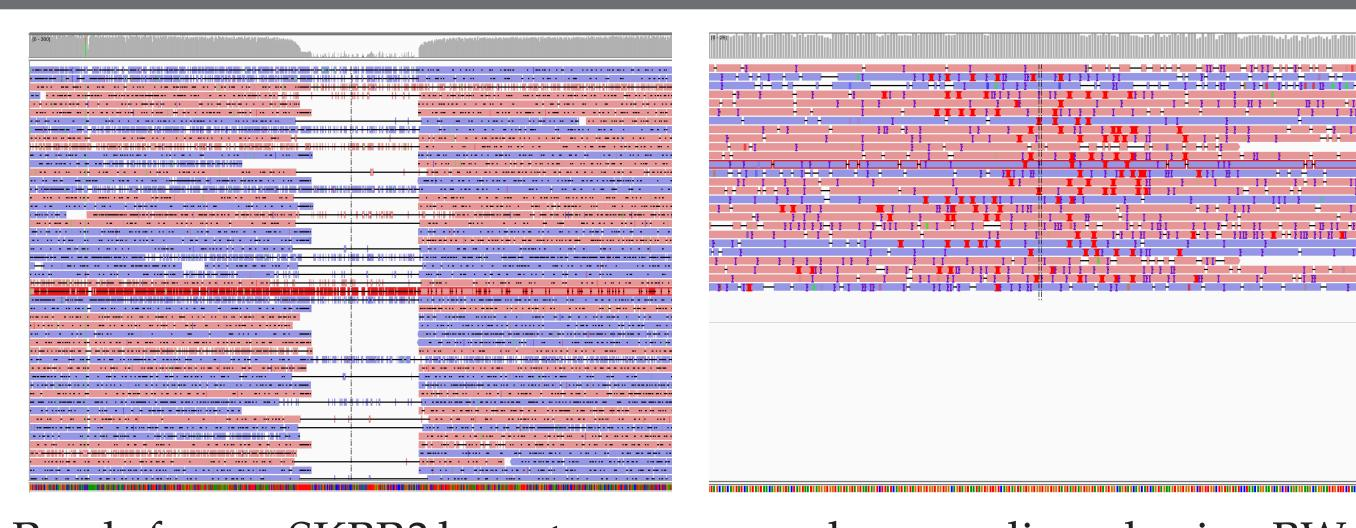
Reads from a SKBR3 breast cancer sample were aligned using BWA-mem 0.7.10 with "-x pacbio". Although, BWA-mem in general produces very accurate alignments, larger **SVs often cause misalignments**. The figure shows example regions containing a 300bp deletion (left) and a 200bp insertion (right).
