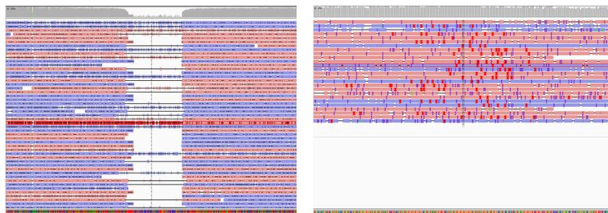
Reads from a SKBR3 breast cancer sample were aligned using BWA-mem 0.7.10 with "-x pacbio". Although, BWA-mem in general produces very accurate alignments, larger SVs often cause **misalignments**. The figure shows example regions containing a 300bp deletion (left) and a 200bp insertion (right).
