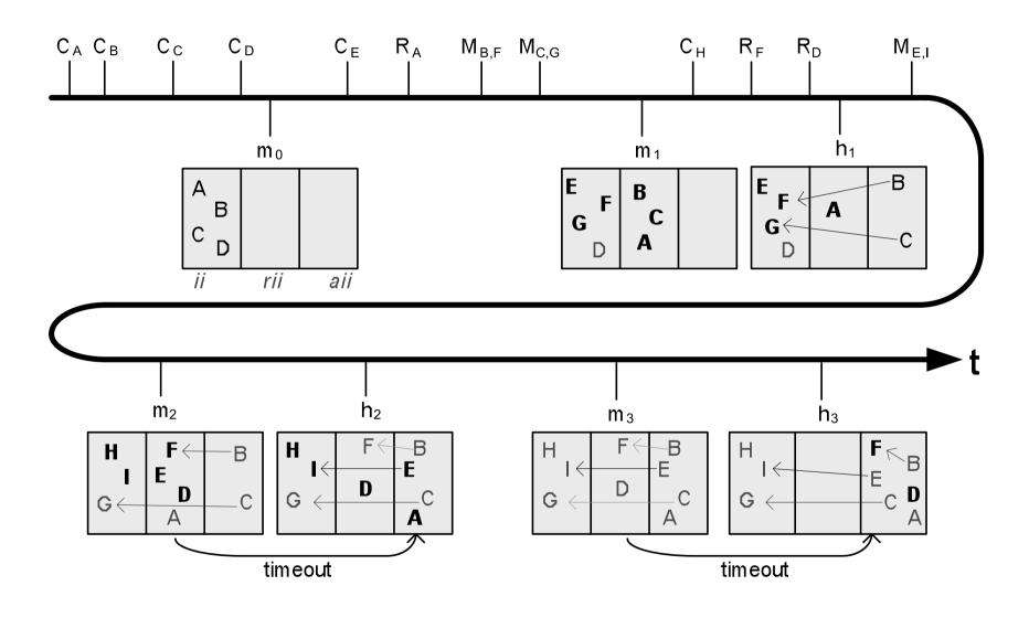
$C_i$ ,  $R_i$  and  $M_{i,j}$  denote *create*, *remove* and *move* events of items i and j.  $m_x$  and  $h_x$  denote *monitoring* and *housekeeping* operations respectively.
