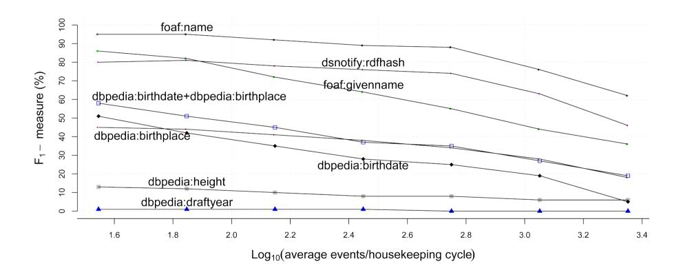
Influence of data source agility and housekeeping frequency on the accuracy of the DSNotify algorithm
