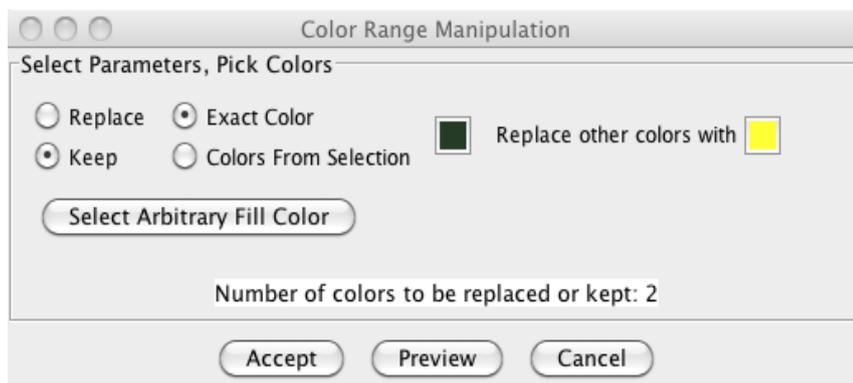
The lower combination of settings allows you to preserve the color green, as shown in the color box, and replace all other colors in the image with yellow. You can also select both colors from the image, or you use a different fill color using **Select Arbitrary Fill Color**.
